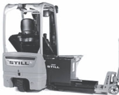
3) Battery change with a standard hand pallet truck, low lift truck or battery change frame
