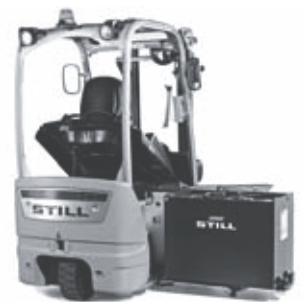
4) On-board roller platform for exchange by hoist
