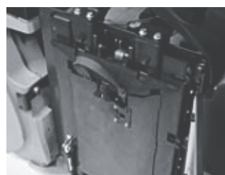
4) On-board roller platform for exchange by hoist
