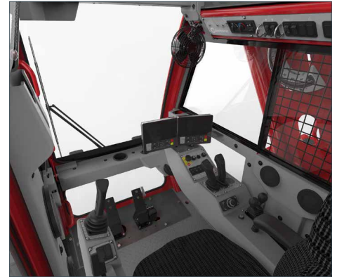
New Wide Body cab with Crane Control System (CCS)
