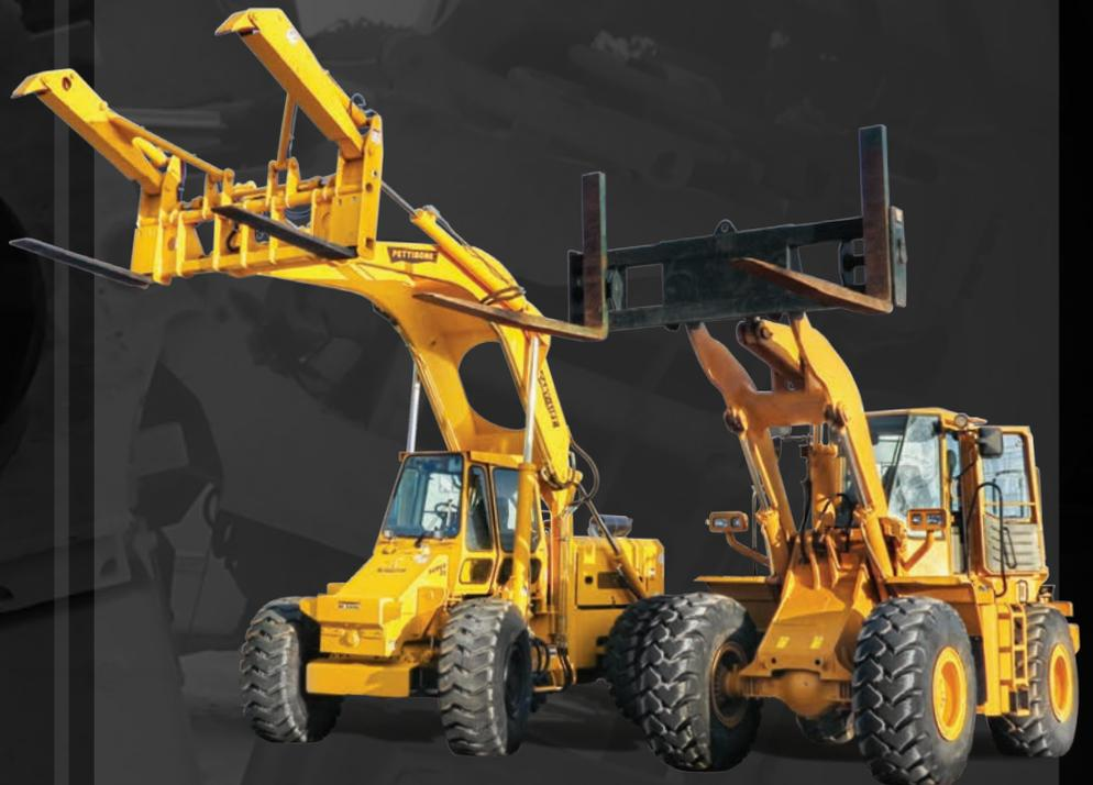
Another issue with a wheel loader’s intended function versus its secondary use as a pipe handler is stability. The articulated steering of a wheel loader is not well suited to making turns while carrying pipe.
