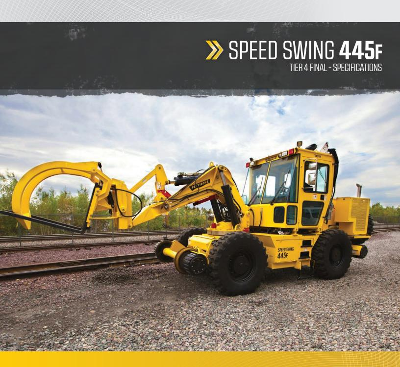
Designed to tackle a variety of rail applications, the Pettibone® Speed Swing™ 445F is a versatile machine that provides the power to lay rails, set ties or clear the path ahead. The unit features a turbo diesel engine and 180-degree boom rotation for enhanced productivity. Offering precise hydraulics, numerous attachments and the ability to work both on and off the rails, the Speed Swing 445F is equipped for any rail task.
